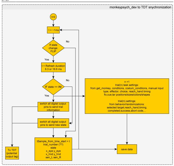
Note that pins are only switched either to send trial information or after a state change (AND after the flip happened!) The idea is that both trial information and state information can be sent via the same channel. Details are described below.
